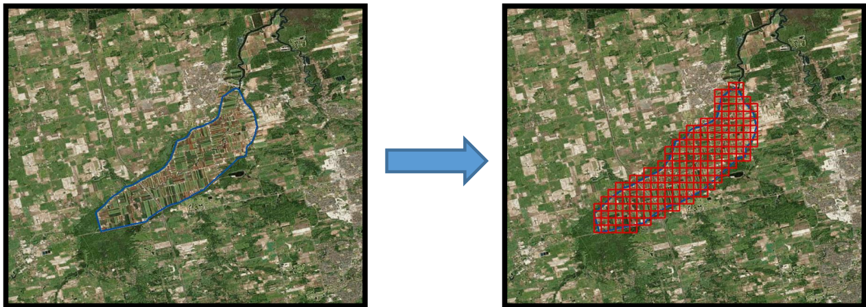
Figure 4-4: Map Algebra, Example of how a raster creates a grid across the study area.
